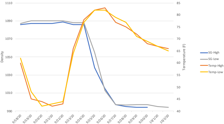
Figure 5: Fermentation kinetics for high and low crop Merlot (In-house data)
