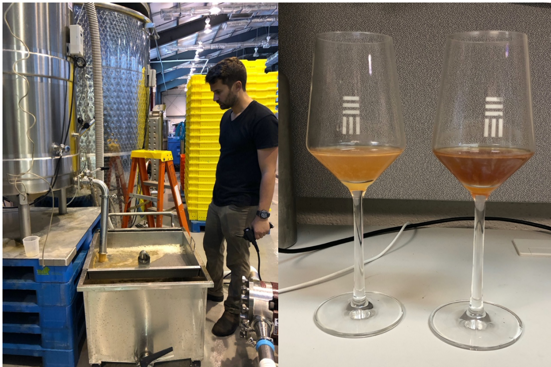
Figure 1: Juice was pumped from the tank through a sump cart to hyperoxygenate. This led to considerable browning.
