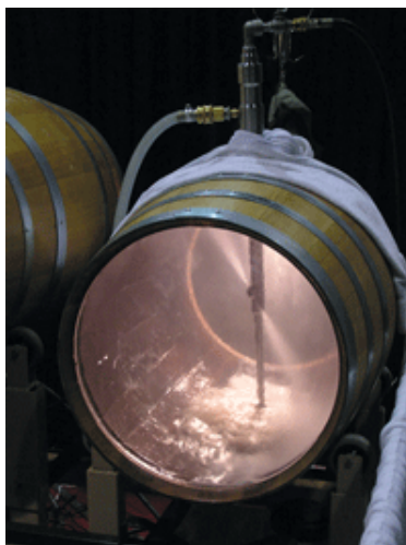
Figure 10.2 – Sideview – High-pressure barrel cleaning wand inside a barrel.
