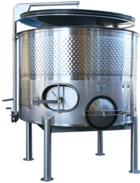
Figure 6.2 – Open Top Fermenter-shallow and wide for improved cap management and temperature homogenization 3
